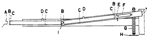
Fig. 1.—Diagram of slit collimating system (scale 10:1): A, X-ray tube exit window; B, mica window; C, tantalum slits; D, vacuum connections; E, Ross filters on slide; F, Geiger counter; G, high precision screw; H, calibrated wheel; I, pivot and sample holder; J, rollers.
